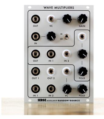
The **middle section** generates a sweep of the odd harmonics (1, 3, 5, 7, 9, 11 and 13th) when a sine wave is applied to its input and the FOLD knob is turned up or a control voltage is swept from low to high. This effect is similar to overblowing a wind pipe closed at one end. A second input is included to allow two signals to be mixed before processing. This module can be used to explore timbral areas beyond the range of ring modulation.
