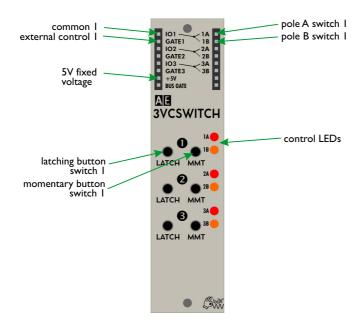
Each switch in this module has three terminals: IOx in the left connectors row, xA, xB in the right connectors row (x represents the number 1...3).
