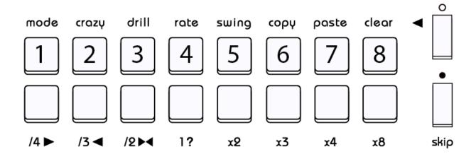
The bottom row of 8 pads apply the tools to tracks 1 to 8 respectively see the next sections for details.
