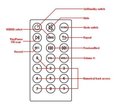
In addition to the panel controls, an infra-red remote control is provided for the USB/SD player which adds some further functions to allow greater control over the media player.
