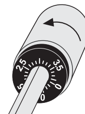
Fig. 6: Stylus pressure adjustment
