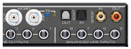
**Word Clock** I/O (BNC): A push switch activates internal termination (75 Ohms). When termination is activated the yellow LED beside the switch lights up.
