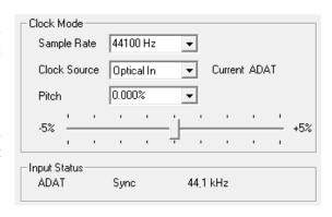
This way, configuring any suitable audio application for digital recording is simple. After selecting the required input, Fireface UC displays the current sample frequency. This parameter can then be changed in the application's audio attributes (or similar) dialog.
