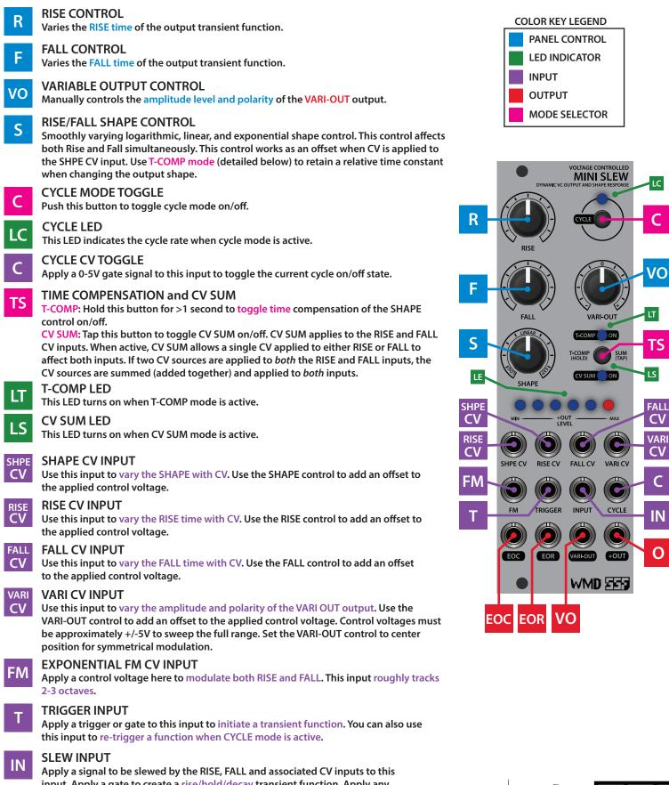
input. Apply a gate to create a rise/hold/decay transient function. Apply any control voltage or audio signal here to dynamically shape the input signal.
